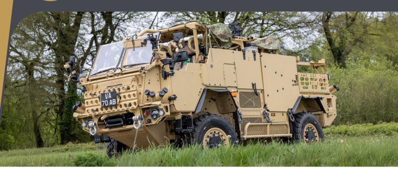
The HMT Extenda is based on Supacat's proven Common Base Platform and adopts a modular approach to enable the users to configure the vehicle to suit specific mission profiles and requirements.
